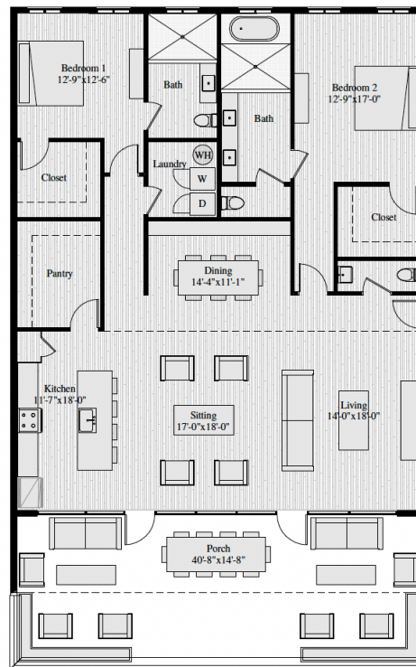
Type F - Penthouse - 2 Bed/2.5 Bath Units 501 & 502 - Level 5 only Total square footage heated/cooled - 2,139 SF Porch - 639 SF
